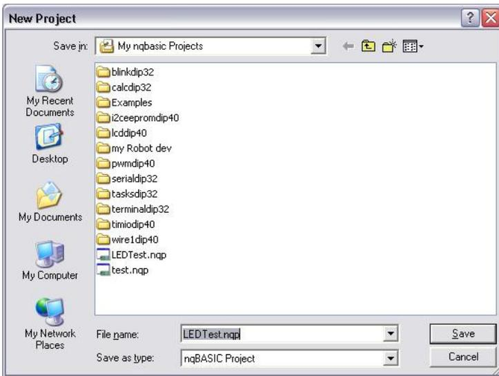
A **NewProject** Window will pop up, showing **LEDtest** as the project name, and will show, by default, that the intended target is NanoCore12 (24 pin DIP). To select a different Target, click the dropdown arrow to reveal the available targets, and select the one you are using.
