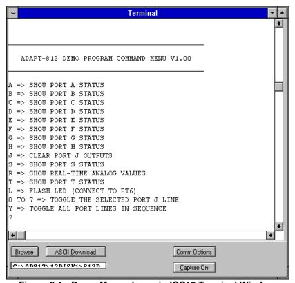
Figure 3.1 - Demo Menu shown in ICC12 Terminal Window
