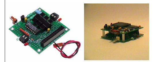
The MicroCore-11<sup>™</sup> Motor Driver Module is one of a range of versatile, low-cost application cards designed for the MicroCore-11<sup>™</sup> 68HC11 microcontroller module.
