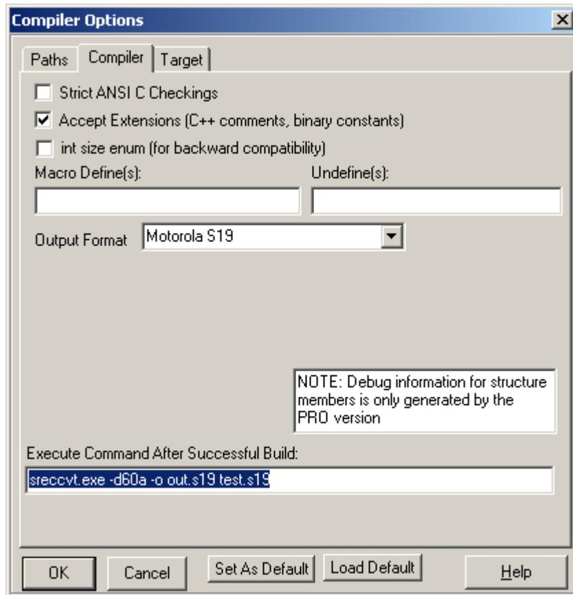
Note that **test.19** is the original S-record and **out.s19** is the file to be uploaded to the MCU.
