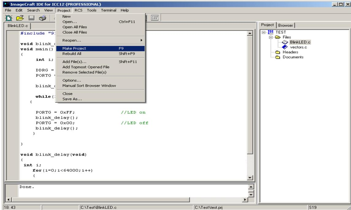
Note the bottom window pane will show messages to display how the build progressed. Any errors, if any, are shown in this window. The build was without error so we can progress to erasing and programming the 912D60/A.
