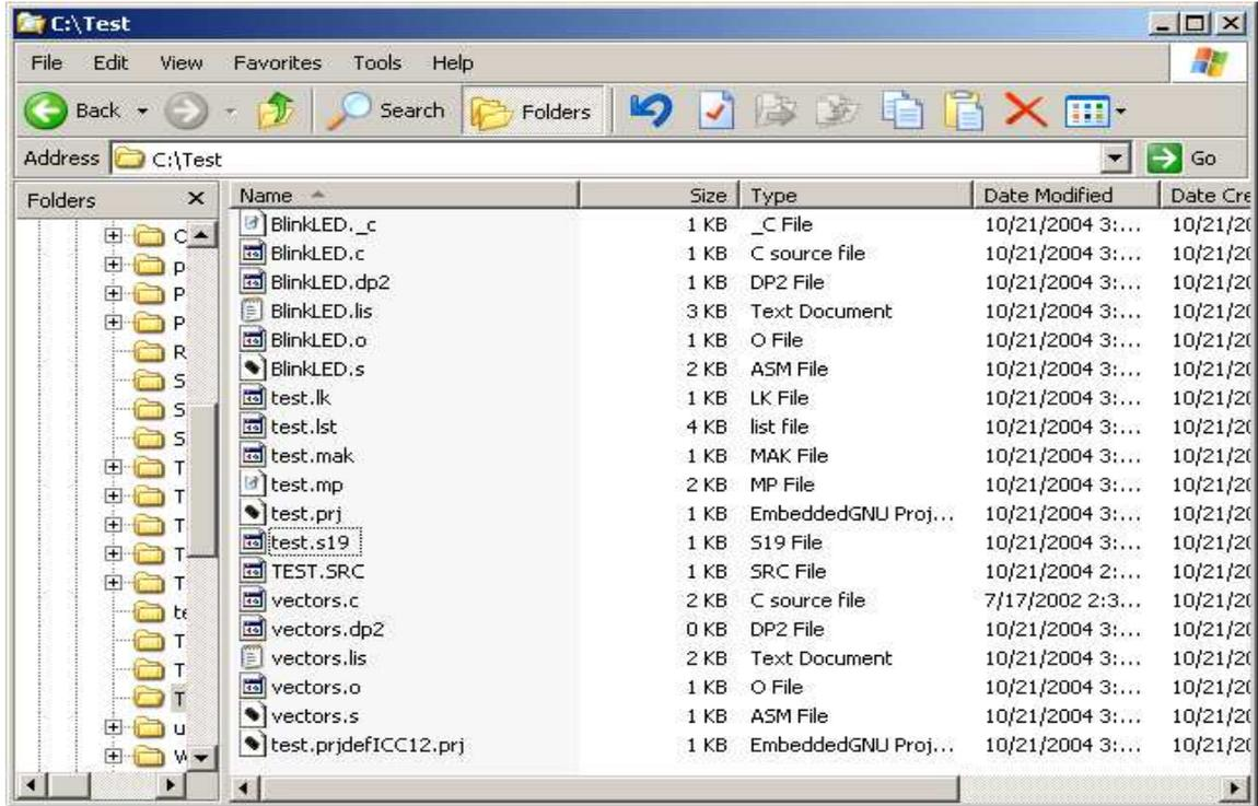
Using WordPad to check the content of **test.s19** file. Note that the S-records are of different lengths.
