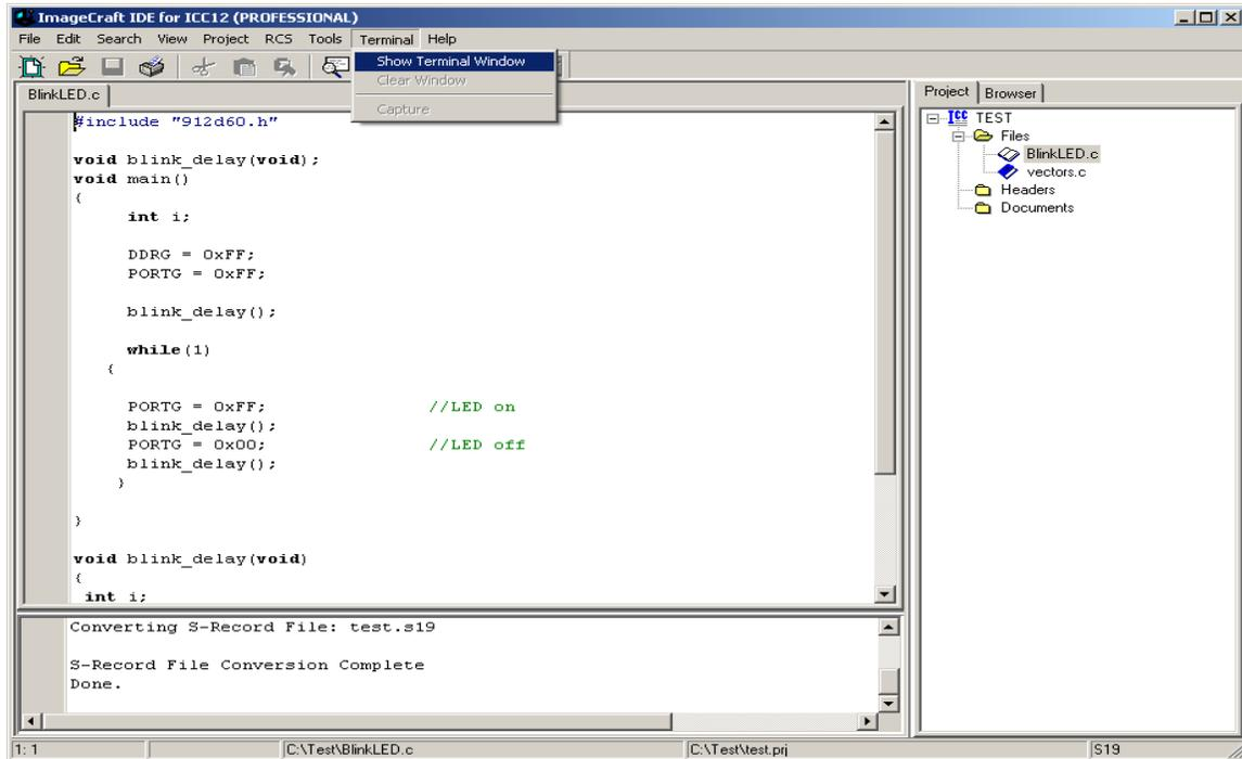
Set the COM port parameters under Tools-Environment Options and then Terminal tab.
