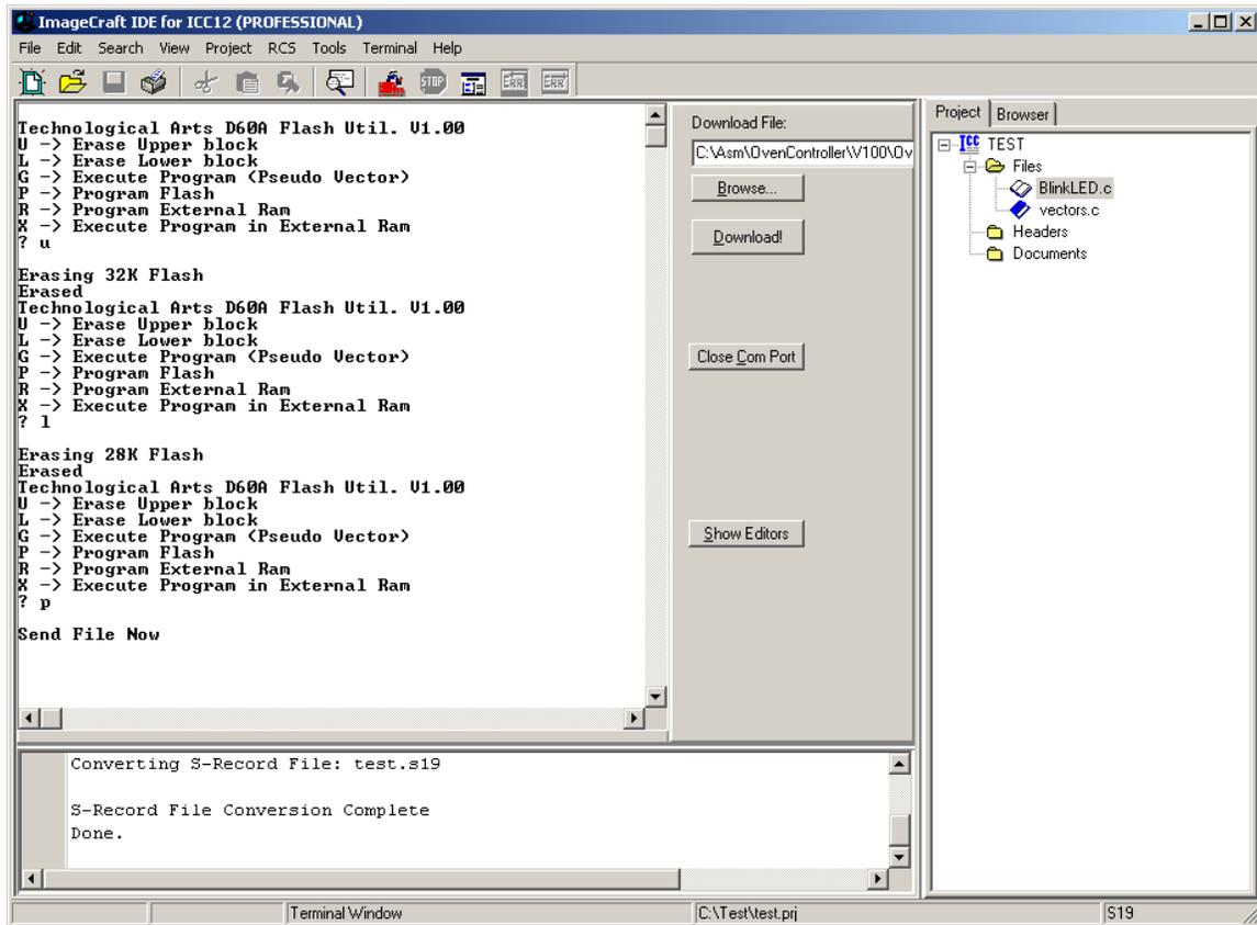
Under the Download File press the Browse button to help locate the **out.s19** file. Select **out.s19** then press the **open** button.
