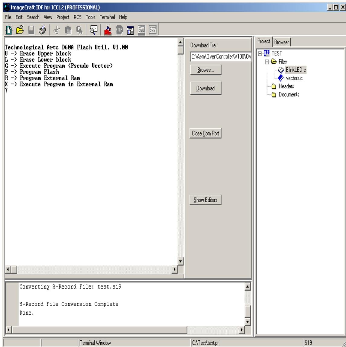
Please note that in the 912D60/A the Flash modules are in 2 locations. One is below \$8000, beginning at \$1000 to \$7FFF (Lower block). The other is at \$8000 to \$FFFF (upper block). The FlashLoader allows one to erase either Lower or upper memory blocks. Since the code starts from \$1000 and the Pseudo vector at \$DFD0, it is important that both blocks be erased.
