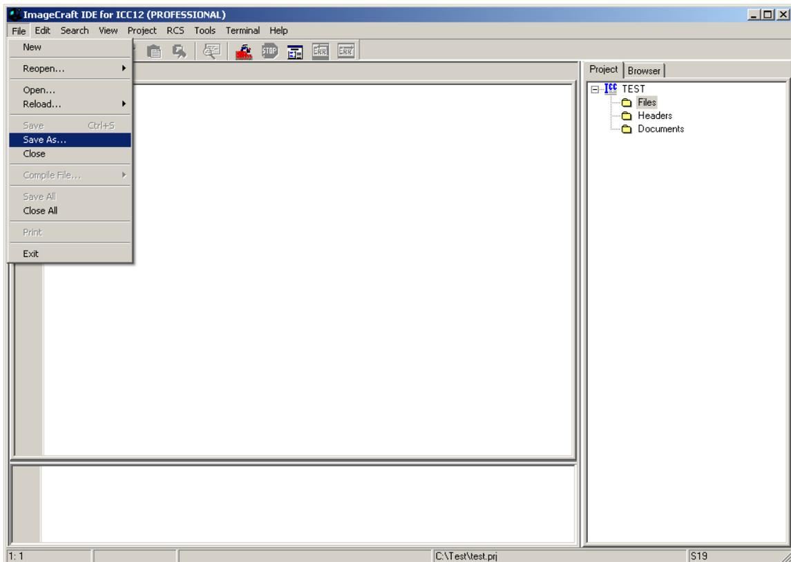
ICC12 will open an explorer window to help save the file. Type BlinkLED.c then press the save button.
