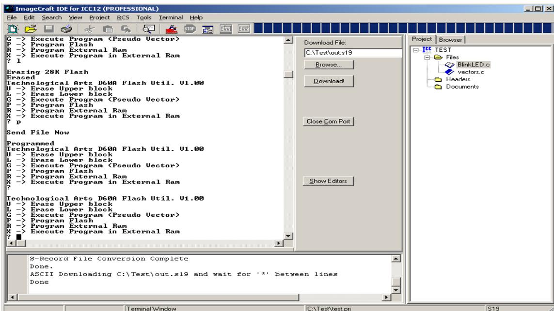
Once file transmit is completed a **Programmed** message will appear on the screen as shown.
