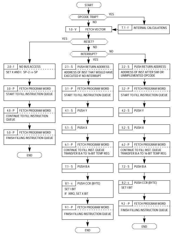
Figure 7-1. Exception Processing Flow Diagram
