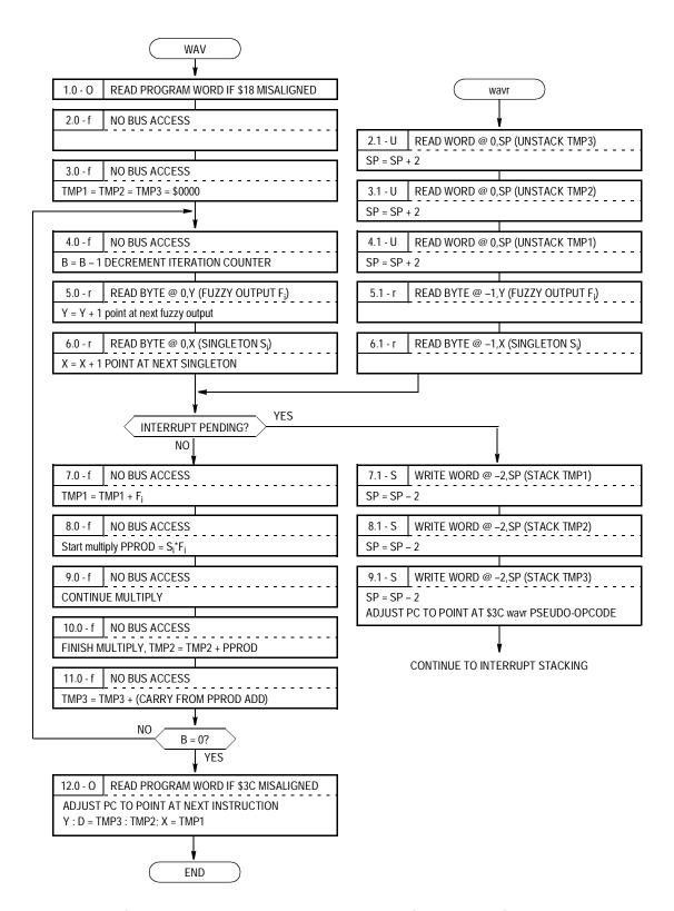
Figure 9-11. WAV and wavr Instruction Flow Diagram
