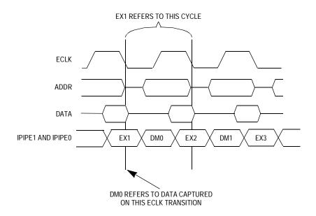
Figure 8-1. Queue Status Signal Timing
