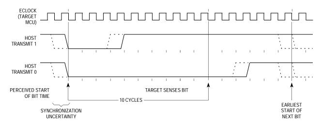
Figure 8-2. BDM Host to Target Serial Bit Timing
