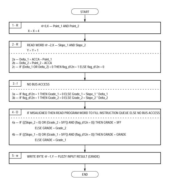
Figure 9-5. MEM Instruction Flow Diagram
