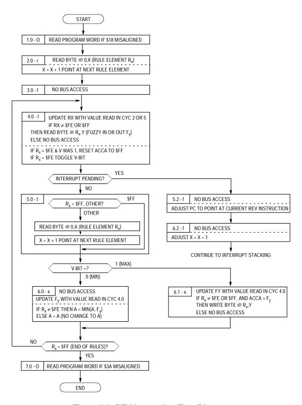
Figure 9-9. REV Instruction Flow Diagram
