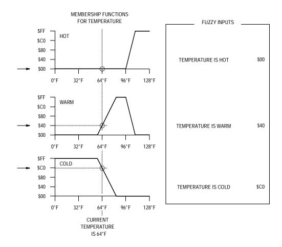
Figure 9-2. Fuzzification Using Membership Functions
