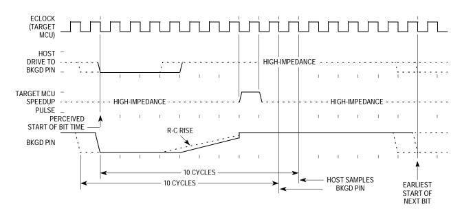
Figure 8-3. BDM Target to Host Serial Bit Timing (Logic 1)
