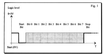
Fig. 1 RS-232 word with 8 Data bits, no parity and one Stop bit, using positive logic and 5V levels
