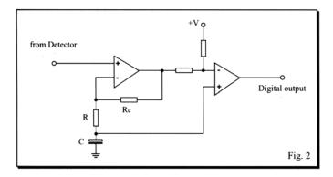
Fig. 2 Schematic diagram of Receiver (LF)
