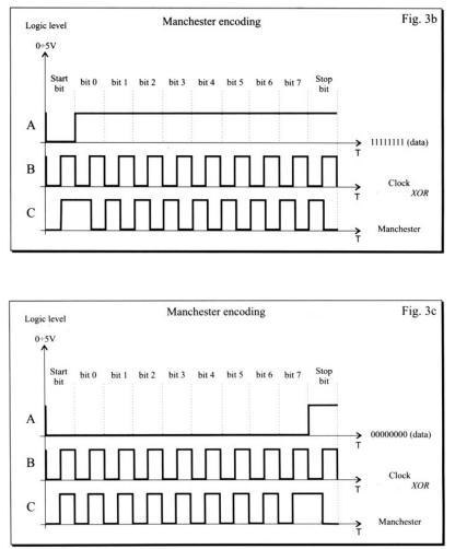
The encoding is simply an exclusive-OR function between the data and a clock frequency of twice the bit rate. This can be carried out either in software, if a microprocessor or microcontroller is generating the data to be transmitted, or using an XOR gate and perhaps a D-type to synchronise the data to the clock frequency if required.
