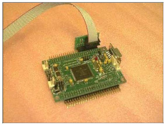
The small circuit board includes a 20 pin connector that fits over the section of pins on H1 of Adapt9S12DP256 that DBUG12 uses to implement BDM out as shown.
